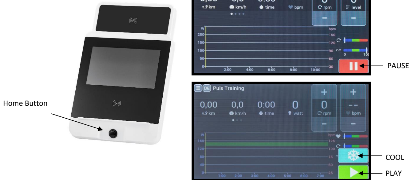
Fig. 2: Monitor view, explaining the button functions, actual view may vary in colour, button assignment is the same.
